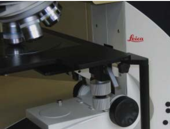
Fast scanning of the entire wafer with the rapid adjustment facility of the manual 6"x6" stage
